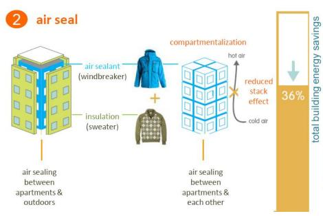
Without air sealing to stop leaks, insulation doesn't work very well. Air sealing is as simple as caulking cracks & holes to the outdoors & between apartments. Not air sealing is like only wearing a sweater (insulation) outdoors on a cold day. You're cold until you put on a wind breaker (air sealing). Air sealing makes the super insulated shell work. It also limits the stack effect, reduces pests & improves indoor air.
