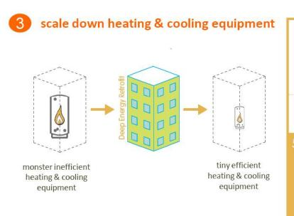
In typical leaky & poorly insulated buildings, big inefficient heating & cooling equipment generally compensates to make residents more comfortable. In contrast, a super insulated & air sealed building requires only a fraction of the energy to heat & cool.
