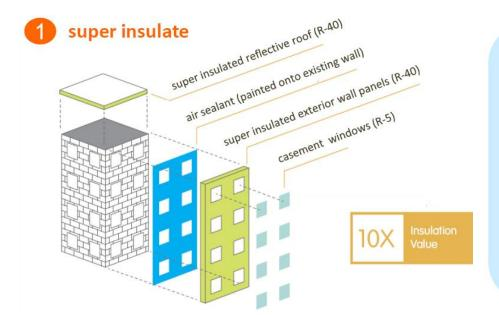
The key difference between a Deep Energy Retrofit & standard energy efficiency renovations is insulation, which at Castle Square will be located on the outside of the building.
