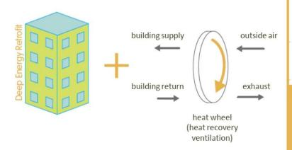
For deeper savings, heat recovery ventilation (HRV) pre-heats or precools incoming fresh air with ventilation air leaving the building (without cross contaminating it). At Castle Square, we were not able to use HRV due to layout constraints & cost issues. Instead, we're using fresh air trickle vents & renovating the existing ventilation system with Aeroseal & CAR dampers
